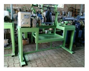
*This machin are suteble for power distribution transformer hv wound coil(squre)winding layer by layer.*
